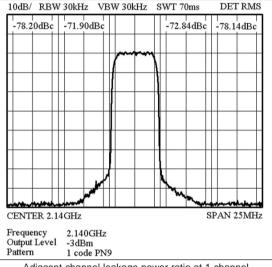
Adjacent channel leakage power ratio at 1 channel
