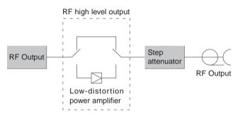
RF high level output option installation diagram
